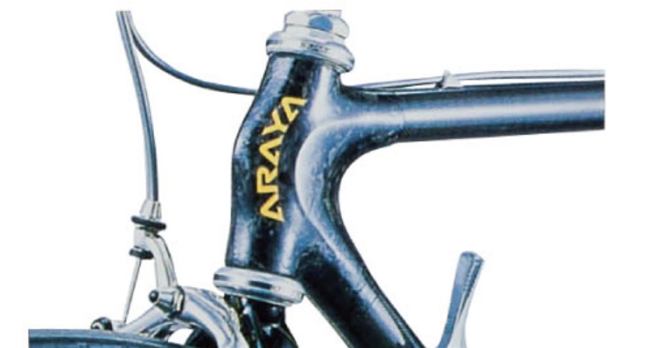
1988 Excella Carbon *Reinforce with Fish-head design
