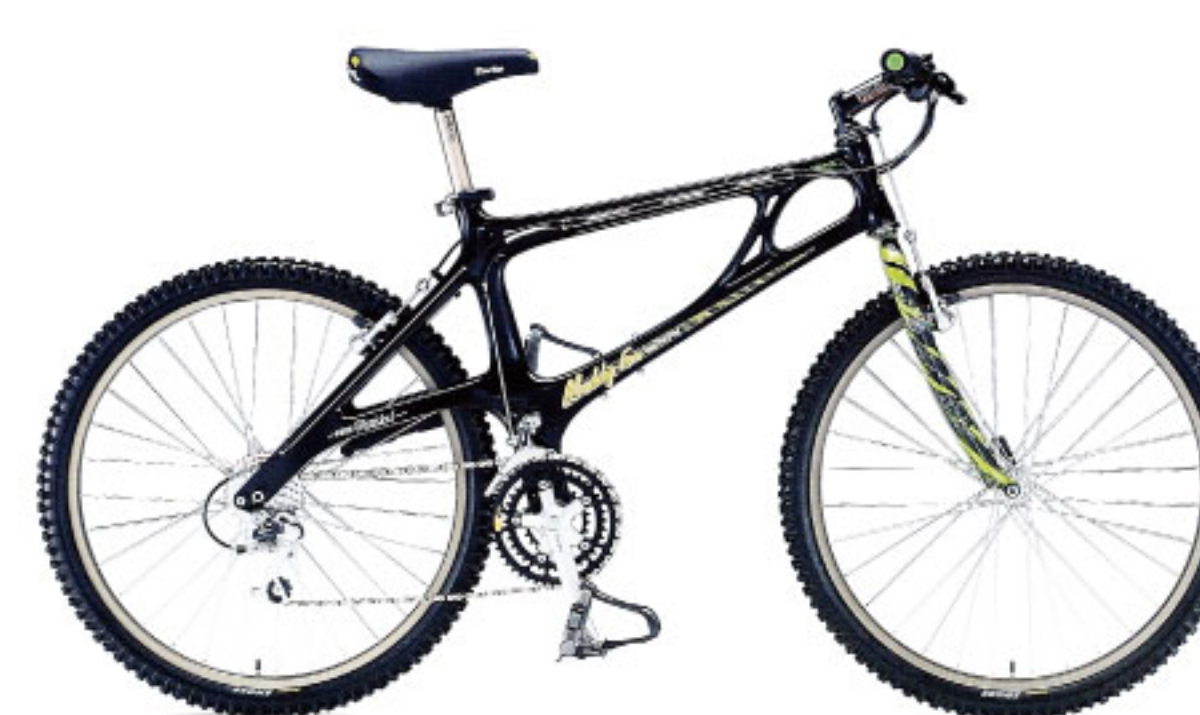
1988 MuddyFox Magnesium *1st Magnesium Frame MTB
